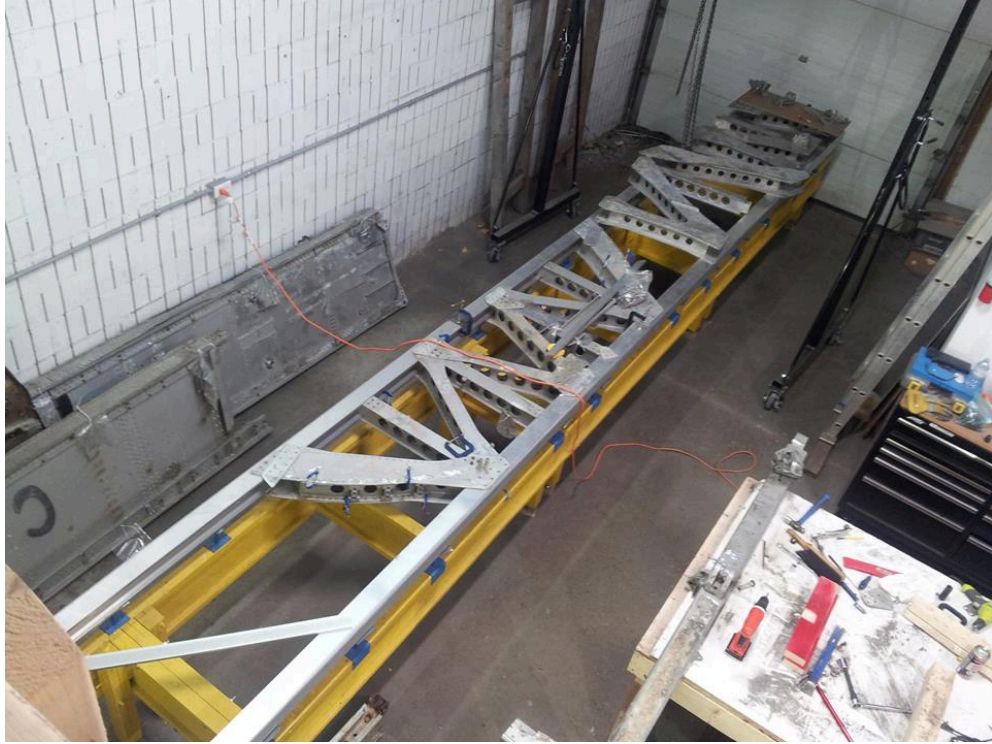
See above our Halifax main spar coming to life at Knox Tech in Ottawa
