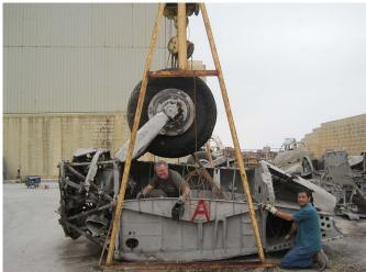
(note: the main wing attachment points to the outer wing panels on the wing rib are still intact and undamaged.)
